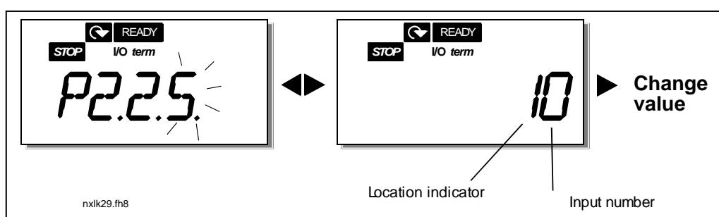
The value of this parameter is formed of the board indicator and the respective input terminal number. See figure above.
