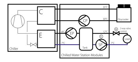
VWF system includes hydronic separator 4-connection tank and evaporator very low pressure and power pump. Evaporator pump works all the time to assure required flowrate on evaporator.
