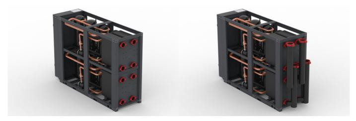
2 cicuit units have totally independent refrigerant circuits. You can collect water from 2 evaporators / 2 condensers by your installation site piping. Or you can order factory build collectors for evaporators and condensers.
