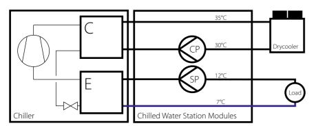
Condenser and system pumps from leading suppliers. Choose high or low pressure or special pump. SPL - Low pressure system pump SPH - High pressure system pump CPL - Low pressure condenser pump CPH - High pressure condenser pump
