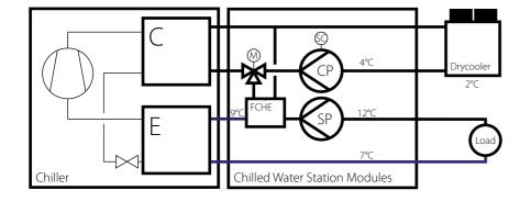
If ambient temperature is lower then system return water temperature the unit will start chilling condenser brine in the drycooler. After this return water will be chilled by brine for free. Compressors will work less time and thus reduce electrical consumption. Unit will work all year around even in th lowest ambient temperatures.
